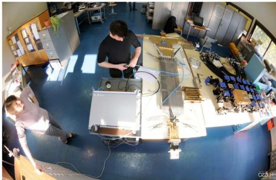
Figure 3. A student is performing a calibration of the Network Analyzer for the Mode Converter measurement.
