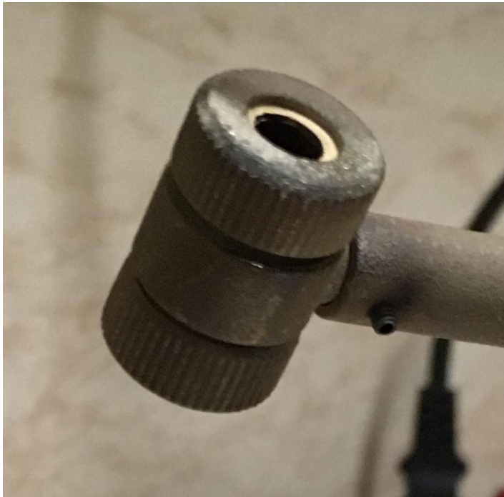
Double tunnel probe at tokamak GOLEM.
