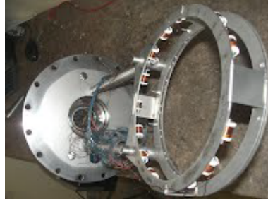
Figure 2: New set of local magnetic field sensors: 16 Mirnov coils circling the plasma column.
