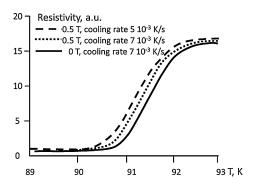
Resistance of a HTS sample vs temperature at different external field and cooling speed.
