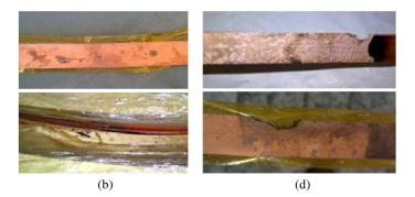
Hot spots (a,b) and arc damaged tapes, (c,d)
