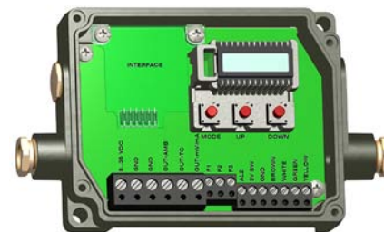
Fig. 31 Opened controller CT-SF02, CT-SF15, CT-SF22 | CTP | CTF-SF15, CTF-SF25, CTH-SF02, CTH-SF10 with terminal connections
