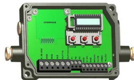
Fig. 32 Opened controller (CTM-1, CTM-2, CTM-3) with terminal connections
