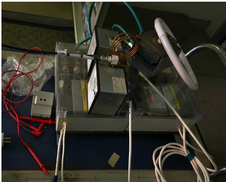
Figure 7: Detection loop (brown copper coil) near magnetron, Fluorescent ring to provide visual emission confirmation and voltmeters besides them.
