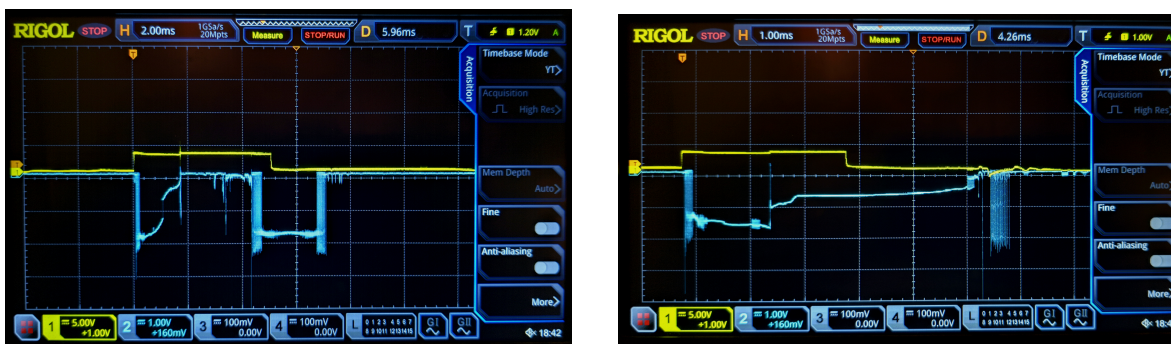
Figure 10: Synchronized oscilloscope measurements: (a) Double pulse in microwave power and (b) Decaying pulse of microwave power. Both show trigger pulse (upper yellow trace) and microwave power output (lower blue trace). The trigger pulse duration is 5 ms.
