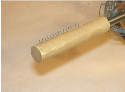
Figure 4. Picture of the rake probe. The insulating probe head is made of Boron Nitride.
